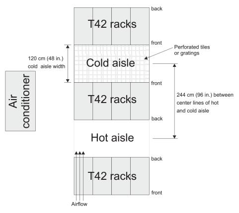
Figure 12. Example of cold aisle/hot aisle rack configuration
